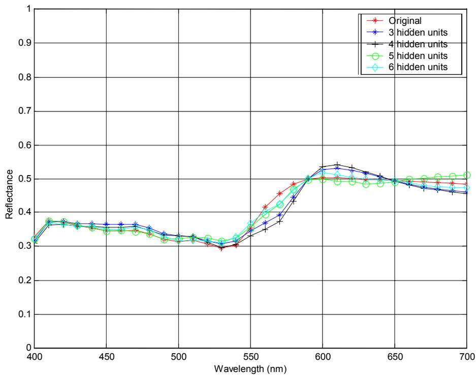
**Figure 2:** Reconstruction of a typical Munsell spectrum using an auto-associative neural network
