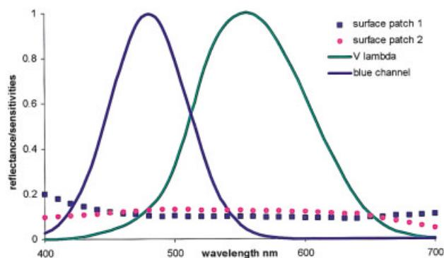
FIG. 1. Reflectance spectra of two hypothetical gray surfaces with spectral reflectance that varies with wavelength.
