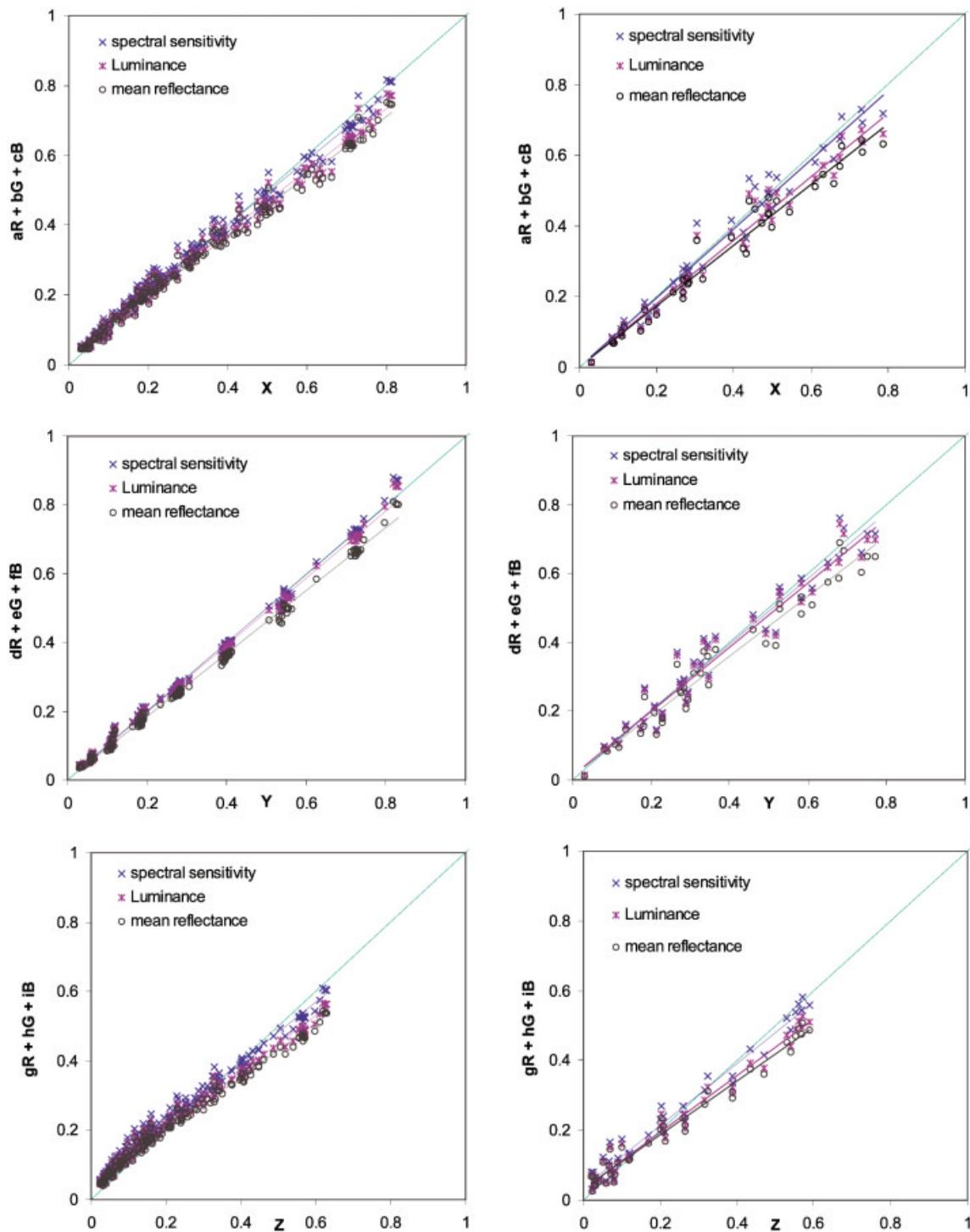
FIG. 4. Correlations for the DC samples (left) and the NCS samples (right) between tristimulus values and linear transforms of camera responses using different linearization techniques. The solid lines show linear regression fits and the dashed shows perfect linearization with a gradient of 1.
