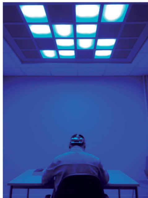
Figure 1 Lighting room showing the position of the participant and the luminaires
