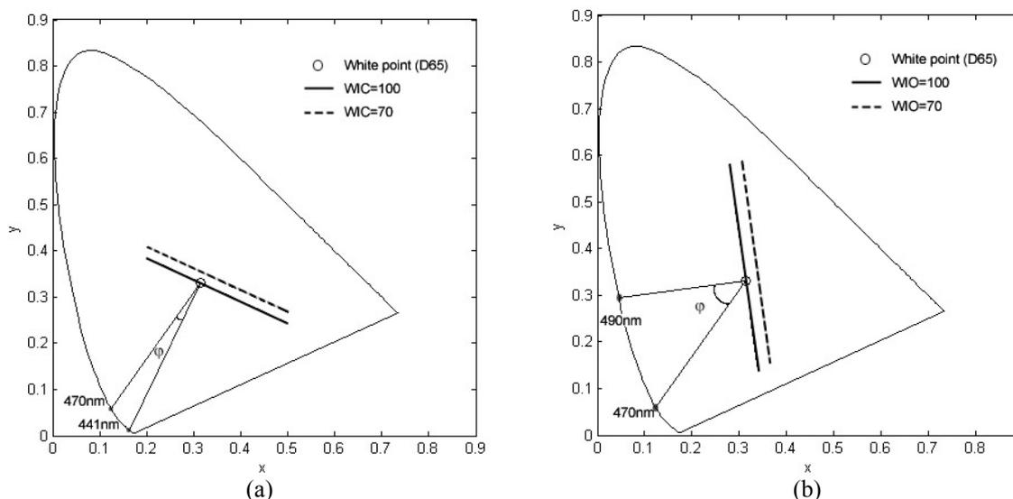
**Figure 2:** The comparison of (a) the CIE Whiteness formula (WIC) and (b) the modified version (WIO) in the CIE chromaticity diagram with illuminant D65 and CIE 1931 2° observer. Based on a dominant wavelength for neutral whites of 470nm the WIC formula can be shown to have a hue preference  $\phi$  of 9.6° whereas the new WIO formula has a hue preference of -45°.
