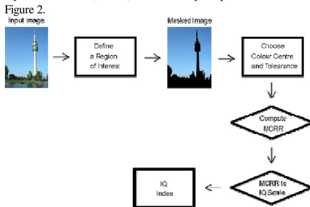
Figure 2. A flowchart of the conceptual process of predicting image quality using memory colour reproduction ratio (MCRR) computing algorithm
