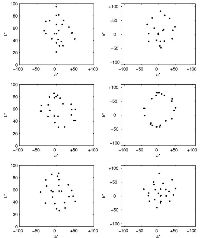
**Figure 7.** CIELAB coordinates under illuminant D65 of the 24 ColorChecker (first row), MAXSUMC (second row), and MAXMINC (third row) samples (for the case where the first sample was selected with maximal spectral variance) plotted in  $L^*$  vs  $a^*$  (left) and  $b^*$  vs  $a^*$  (right) diagrams.
