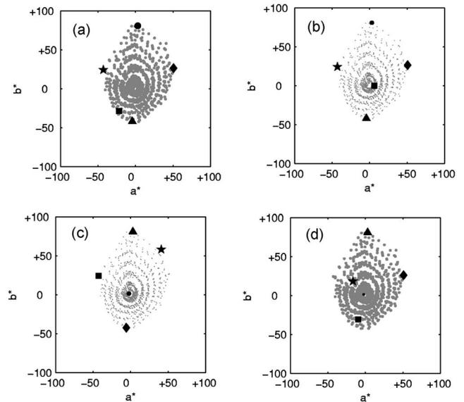
**Figure 3.** Diagrammatic representation of the selection sequence (in order, large circle, triangle, diamond, star, and square) for MAXSUMC [(a) and (c)] and MAXMINS [(b) and (d)] methods where the first sample was selected with greatest [(a) and (b)] or smallest [(c) and (d)] spectral variance.
