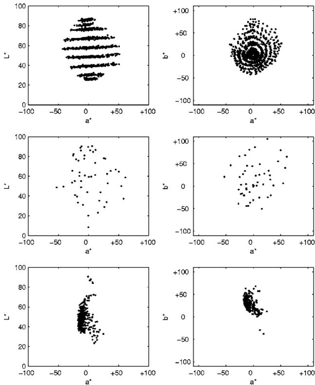
Figure 5. CIELAB coordinates under illuminant D65 of 1269 Munsell (top), 50 selected Natural Color System (middle), and 494 natural (bottom) samples plotted in  $L^*$  vs  $a^*$  (left) and  $b^*$  vs  $a^*$  (right) diagrams.
