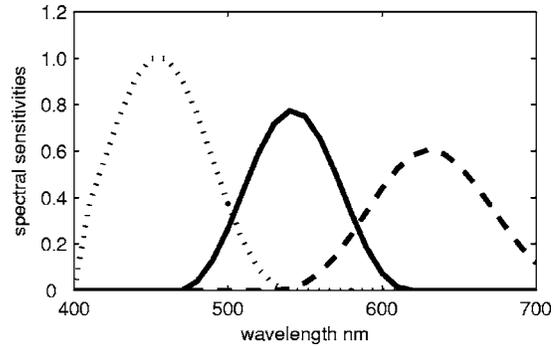
Figure 4. Estimated camera spectral sensitivities (blue channel, dotted line; green channel, solid line; red channel, dashed line) of an Agfa StudioCam: estimation by Chen *et al.* (see Ref. 23).
