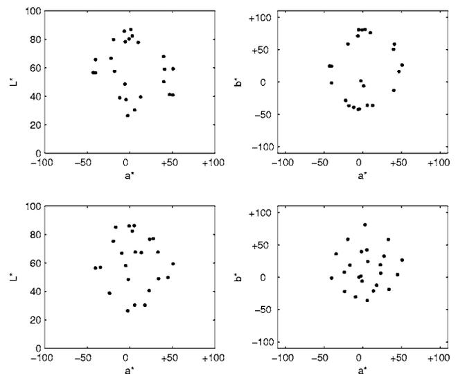
**Figure 8.** CIELAB coordinates under illuminant D65 of the 24 MAXSUMC (upper row) and MAXMINC (bottom row) samples (for the case where the first sample was selected with minimal spectral variance) plotted in  $L^*$  vs  $a^*$  (left) and  $b^*$  vs  $a^*$  (right) diagrams.
