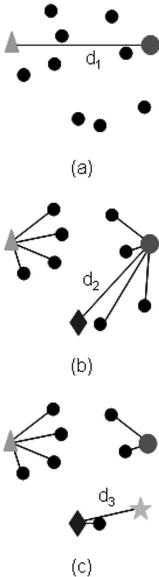
**Figure 2.** Illustration of the MAXMINS method with the first selected sample (large circle) and (a) the second selected sample (triangle) chosen such that it is maximally distant from its closest neighbor in the selected samples; (b) the third selected sample (diamond) chosen such that it is maximally distant from its closest neighbor in the selected samples; and (c) the fourth selected sample (star).
